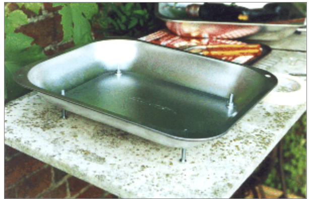
4. The support bolts for the drip tray
