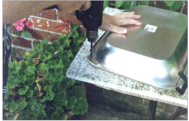
2. Drilling the holes for the locating bolts
